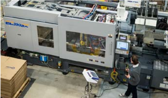
Polyfab's cutting-edge production facility operates the ComoNeo and CoMo Injection process monitoring systems as well as cavity pressure sensors from Kistler
