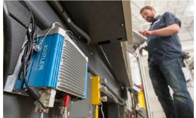
The technicians receive detailed real-time information about the cavity pressure profile thanks to ComoNeo (All photos: Kistler)
