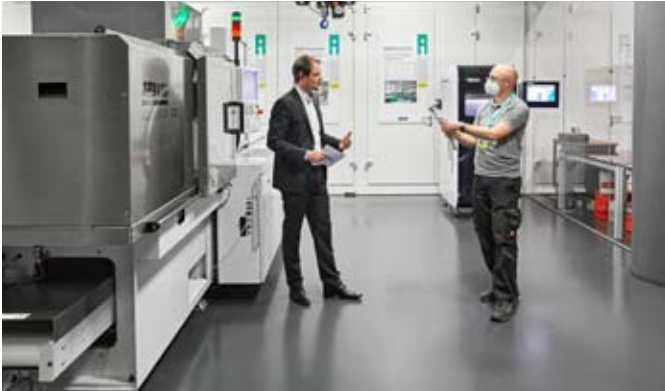
"Live Breakout Box" cleanroom: Arburg expert Sven Kitzlinger, Senior Application Manager Medical, answered questions from the participants about cleanroom technology and presented interesting features directly beside the injection moulding machine that was producing needle holders for insulin pens in a live demonstration
